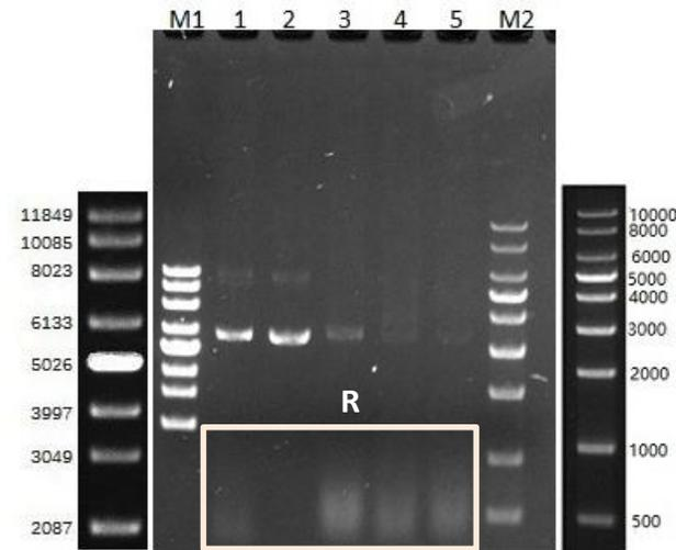
**Agarose gel electrophoresis (AGE):** obvious decrease of RNA content through 1<sup>st</sup> purification step.
